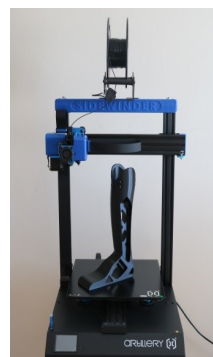
Fig. 11. 3D printing ultimate below-knee prosthetic leg
