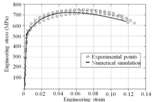
**Fig. 8.** Comparison of engineering stress- strain in tensile test loading-unloading
