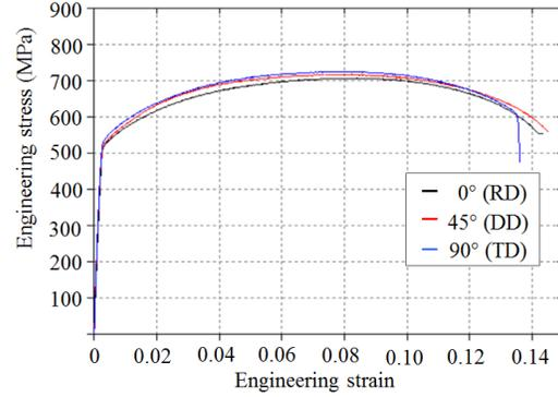
**Fig. 1.** Engineering stress-strain curves
