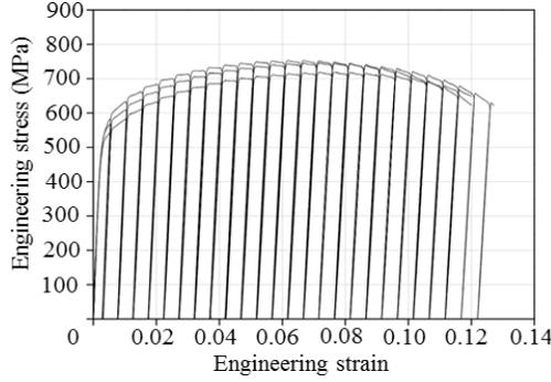
**Fig. 2.** Engineering load-unload curves
