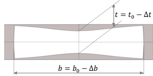
**Fig. 3.** Illustration of necking of a rectangular specimen
