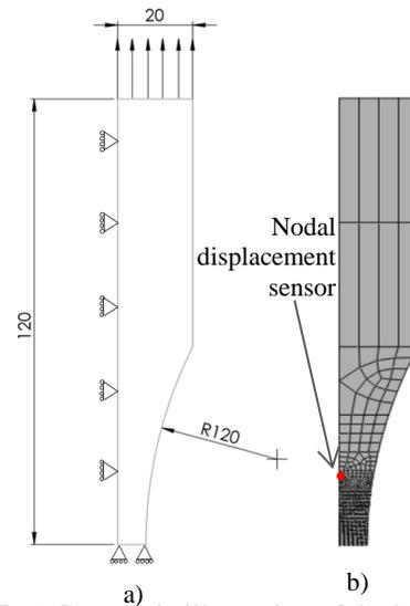
**Fig. 7.** a) Geometric illustration of the hourglass flat specimen (dimension in mm), b) FE mesh of the tensile test.
