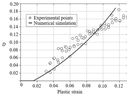
**Fig. 9.** Numerical comparison of the damage evolution versus plastic strain for DP590 steel
