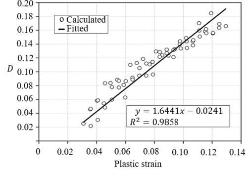
**Fig. 6.** Linear regression procedure to obtain damage resistance  $S$
